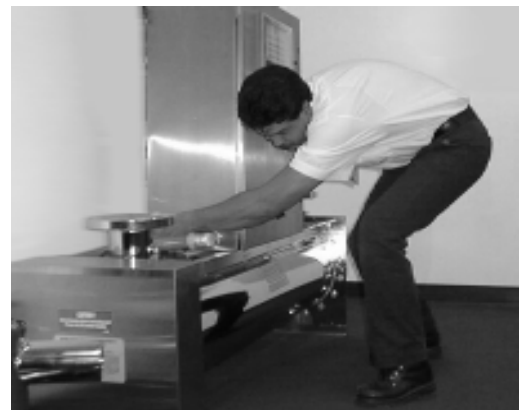
Fixed enclosure: Remove the air filter by feeling for it beneath the enclosure and then pulling it out towards you.
