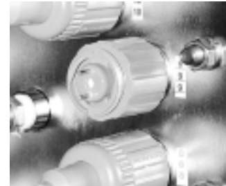
UV lamp securely inside locking mechanism
