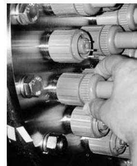
Screw the lamp socket cap into place
