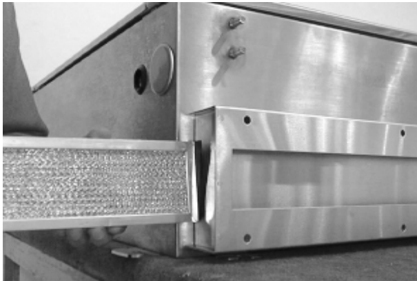
Remote enclosure: Removing the filter (view from underneath the enclosure)
