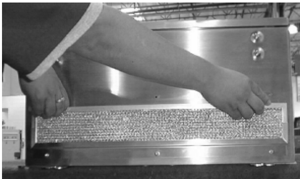
Fixed enclosure: The air filter is located underneath the enclosure cabinet and must be located by touch because of the close proximity of the treatment cylinder and cabinet.
