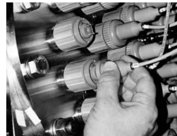
Secure lamp socket connector to lamp
