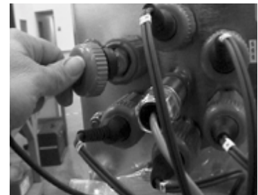
Secure lamp socket connector to lamp
