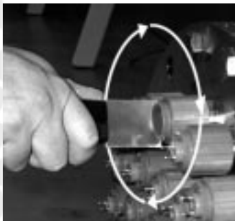
Rotate compression nut clockwise onto the threaded stainless nipped end plate with compression nut tool
