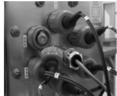
Lamp socket ID number on end plate
