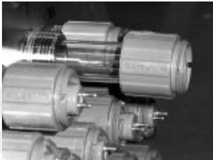
Compression nut assembled on the quartz sleeve
