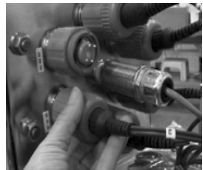
Screw the lamp socket cap into place
