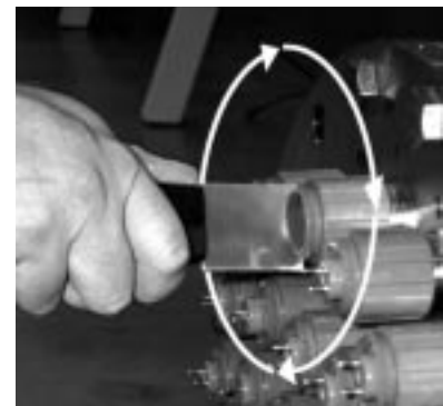
Compression Nut Tool - Rotate clockwise onto the threaded stainless nipped end plate with compression nut tool
