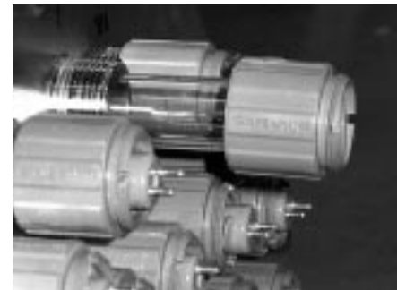
Compression nut assembled on the quartz sleeve
